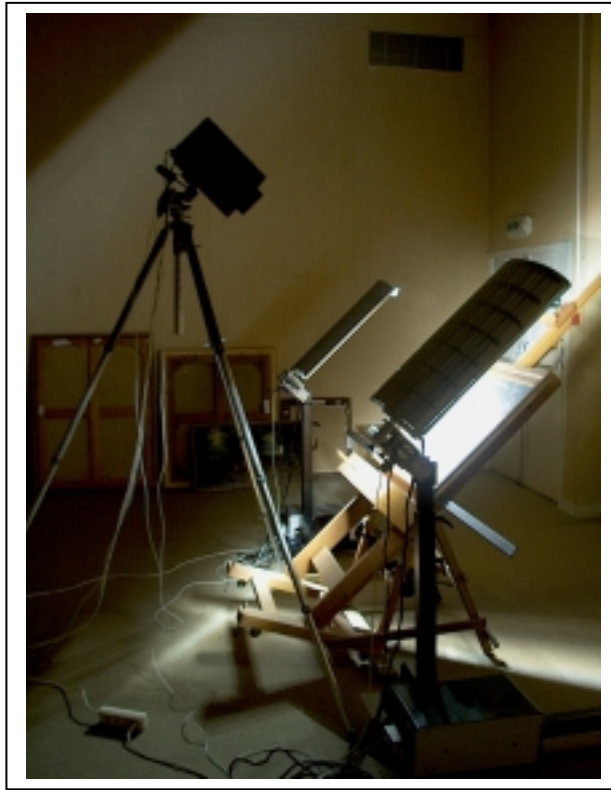
fig. 3 : two Jumbolux linear beam lights operating synchronically with the camera
