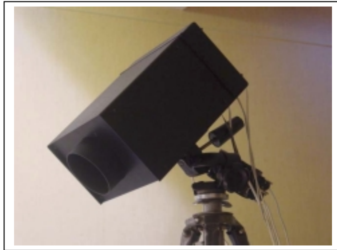
fig. 4 : the Jumboscan high definition camera
